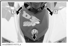
Step 1: Pull front tab from grommets Step 2: Lift cover to remove
